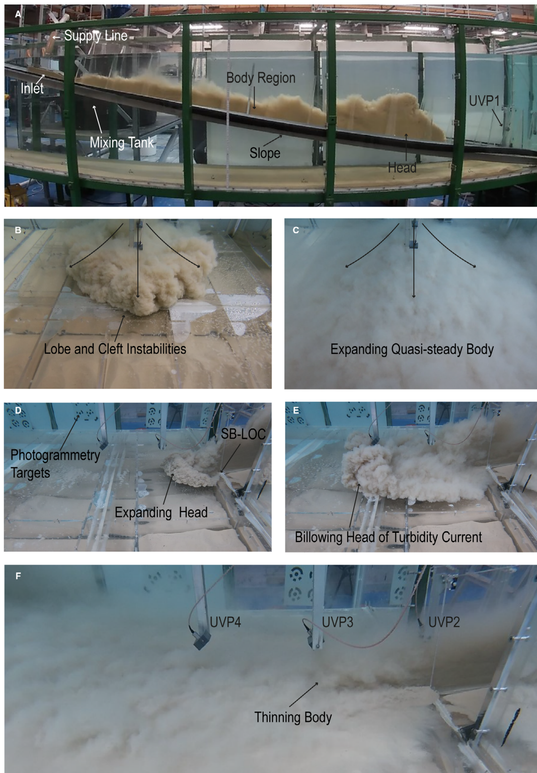
Fig. 4. (A) Formation of the high-density turbidity current (HDTC) head and quasi-steady body region along the confined, sloping channel with flow direction being from left to right, (B) symmetrical radial expansion of the HDTC head downstream of the SB-LOC, (C) expansion of the HDTC body region downstream of the SB-LOC, (D) side on view of the HDTC head expansion 0.25 s after exiting the SB-LOC, (E) side on view of the radially-expanding HDTC, 2.5 s after exiting the SB-LOC, (F) side on view of HDTC body collapse downstream of the SB-LOC. (note the absence of an internal hydraulic jump immediately downstream of the SB-LOC).
