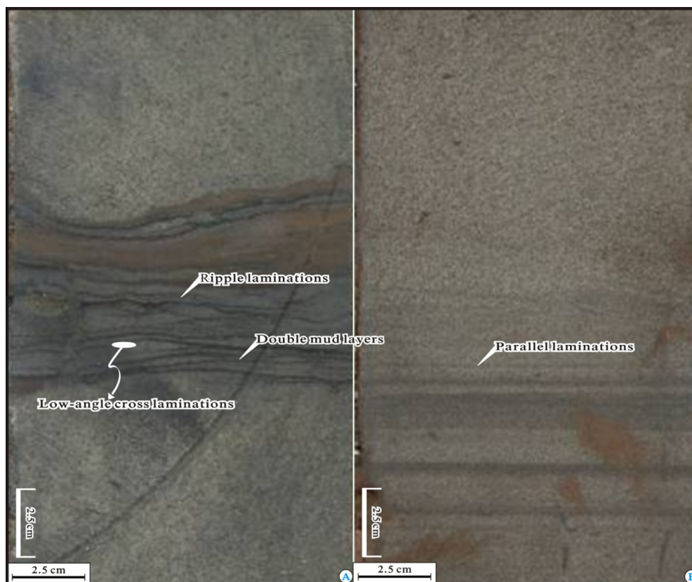
Fig. 5. (Panel A) Core examples of fine-grained sandstones displaying ripple lamination, mud-offshoots, double mud layers, and low-angle cross-lamination. (Panel B) Core examples of parallel laminations seen in ungraded sand facies.
