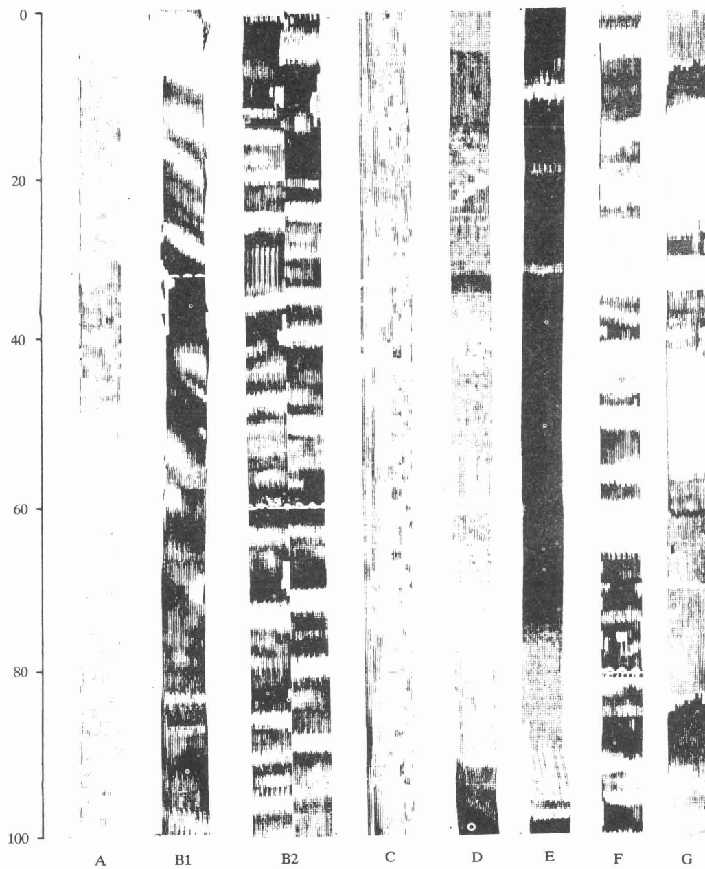
Fig. 4. Characteristic FMS images of volcaniclastic facies: A, debrisites; B, slumps; B1 microfolds (recumbent); B2, microfaults; C, massive structureless sandstones; D, volcaniclastic turbidites; E, calcareous volcaniclastic turbidites; F, pelagites; G, bioclastic turbidites.
