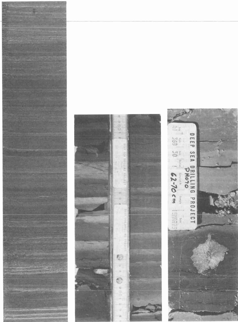
FIG. 10. Examples of redeposited sediments and sedimentary structures associated with 'black shale' facies in DSDP drillholes.
